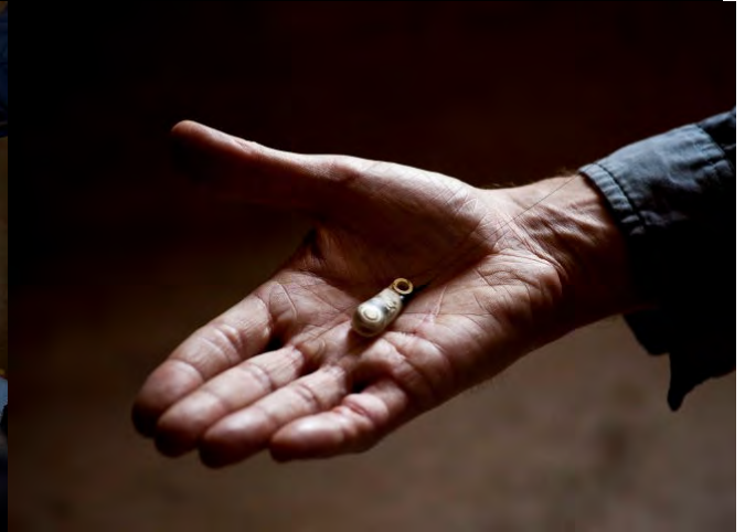
Photo 6. Ear tag transmitter (dummy) coated in dental acrylic, with NiTi antenna.
