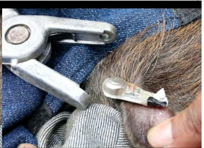
Photo 24. Fitted ear tag transmitter G prior to smoothing off the sharp end of the shaft.
