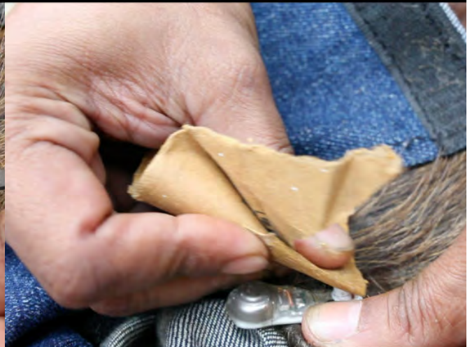
Photo 26. Sanding down of the cut end of the shaft of ear tag transmitter G to provide a smooth flat surface.
