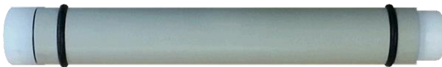
Figure 3: A C-POD static passive acoustic logger (Chelonia, 2015)
