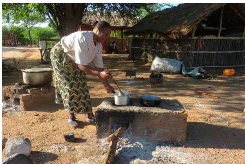
Mama Danieli demonstrating the use of the mud stove, which can cook two meals simultaneously, while only slowly burning one piece of wood
