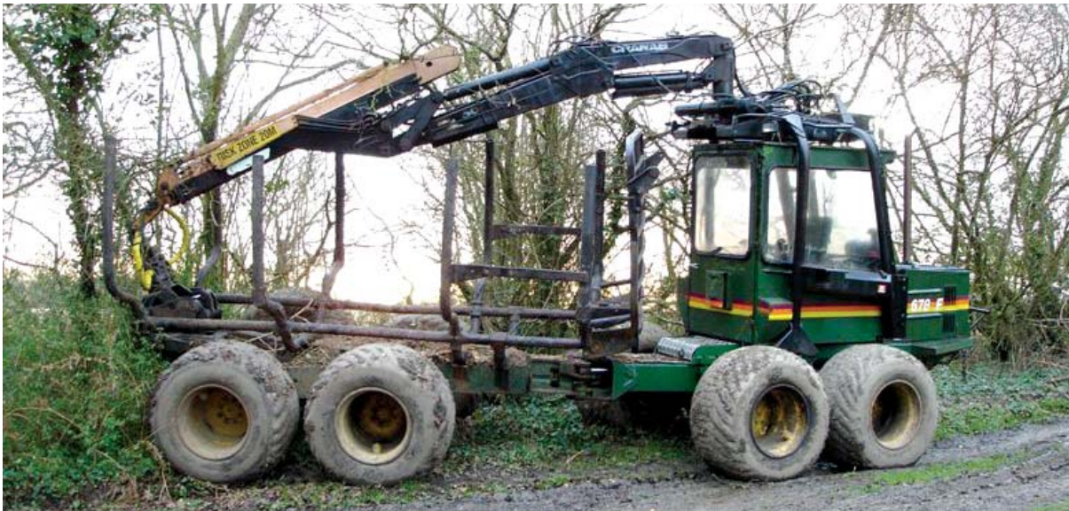
A forwarder is a 6 or 8 wheel articulated machine used to transport logs, which have been cut to prescribed lengths, from the forest floor to a stacking area alongside the forest road, ready for uplift by timber lorries.
