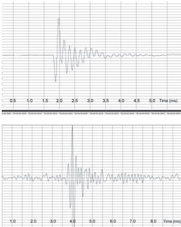
**Fig. 5.** Acoustic patterns produced by biting of *Lucanus cervus* (upper graph) and the lesser stag beetle, (*Dorcus parallelipedus*) larvae.
